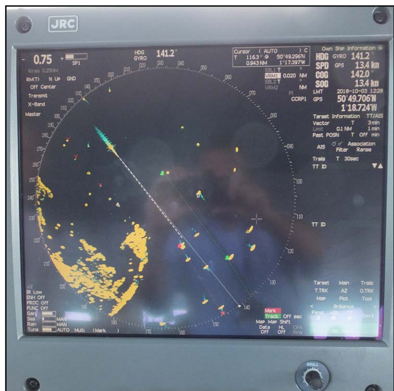
Figure 15: Radar picture offset (approaching Calshot Spit, not in Cowes Harbour)
